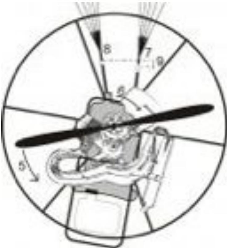
If the engine acts with force on the propeller, the propeller will react with equivalent force. If the prop rotates to left (5), the torque effect will rotate the paramotor to the right (6). The whole paramotor will yaw to the right, mostly with the pilot as well. One side of the paraglider is more loaded and pulled down (9). **The paraglider will have the tendency to turn and is not capable of straight flight without pilot input.**
