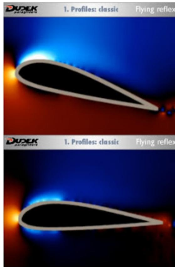
The airflow is most important above the upper wing surface because this is the place where the most of the lift force is generated. The lift force in our case is caused by the lower pressure on the upper part of the airfoil (blue area). The brighter the blue, the lower the value of the pressure. It makes the pressure difference between the upper and lower part of the wing bigger.
