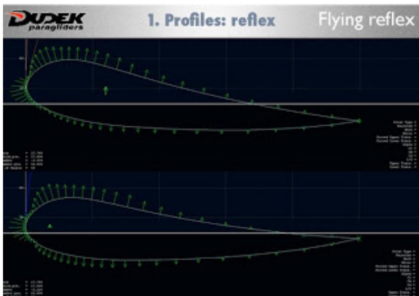
This picture shows the reflex airfoil flying on high (upper picture) and low (lower picture) angle of attack. The arrow inside the airfoil shows how the center of pressure moves forward when the angle of attack is decreased.
