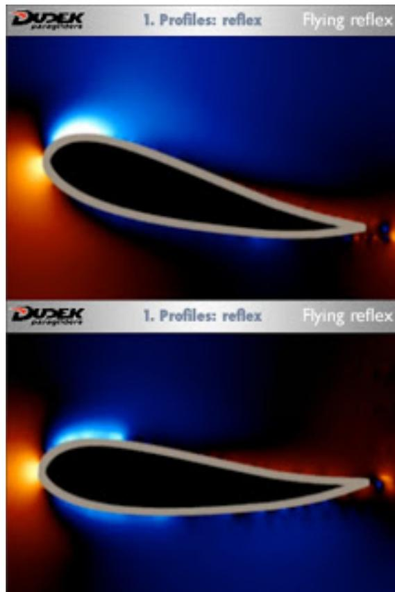
In the case of the reflex airfoil we can see that even though the angle of attack decreased, the center of the pressure did not move backwards. This makes the wing resistant to deformations and collapses. The pressure to 'keep the wing open' is always there.
