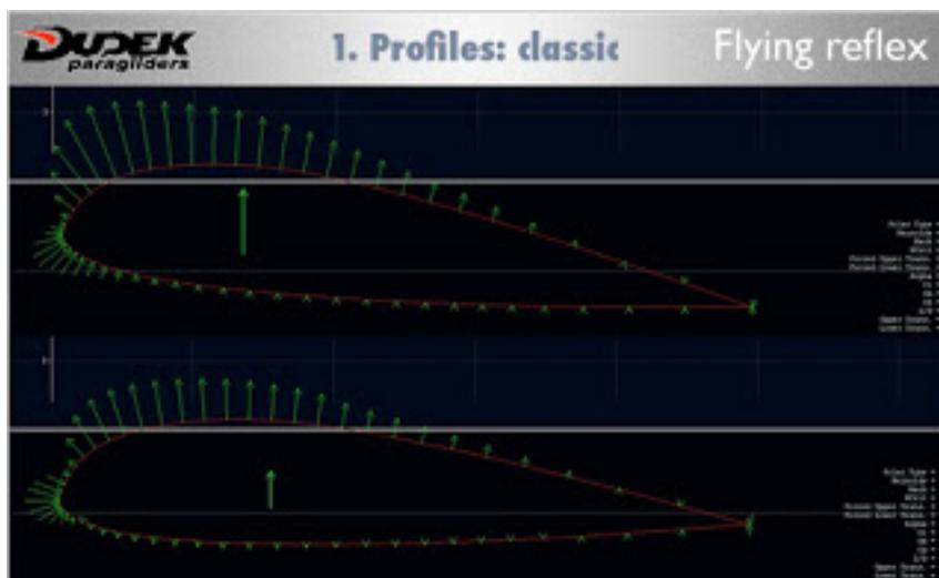
The top picture shows the wing flying on a high angle of attack. The lower picture shows the airfoil on a small angle of attack. The arrows show the pressure distribution along the airfoil and the arrow 'inside' the airfoil shows the magnitude of the lift force and its attachment point (the center of pressure). You can see that when lowering the angle of attack the point of pressure is moving backwards.
