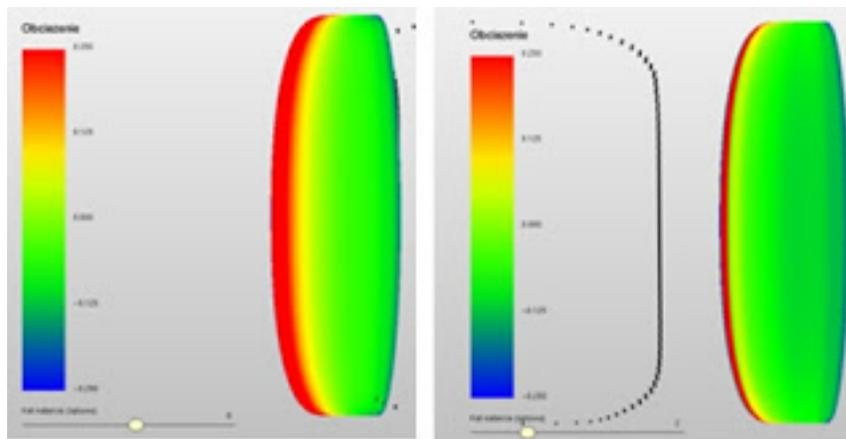
In the above picture we can see the lift force distribution on the reflex wing without speedbar (angle of attack 6 degrees) on the left hand side and with full speedbar on the right hand side (angle of attack 2 degrees).
